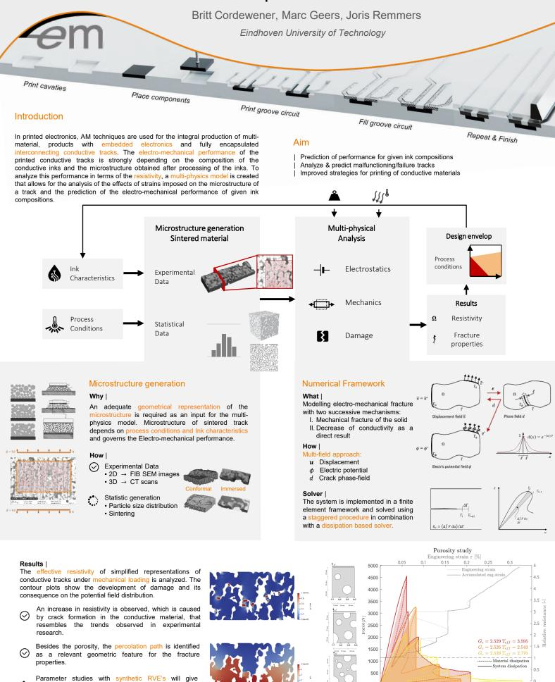
Parameter studies with synthetic RVE's will give insights in the effects of sintering times and particle size distributions.
