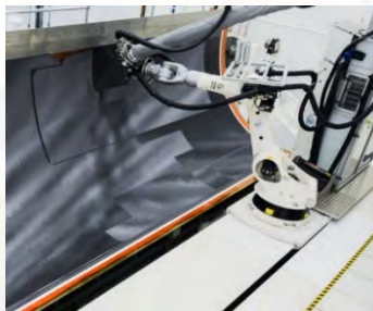
Figure 1: Robot system to produce an 8-meter-long thermoplastic composite fuselage section [1].
