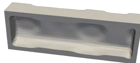
(b) Hollow centre of the torsion beam
