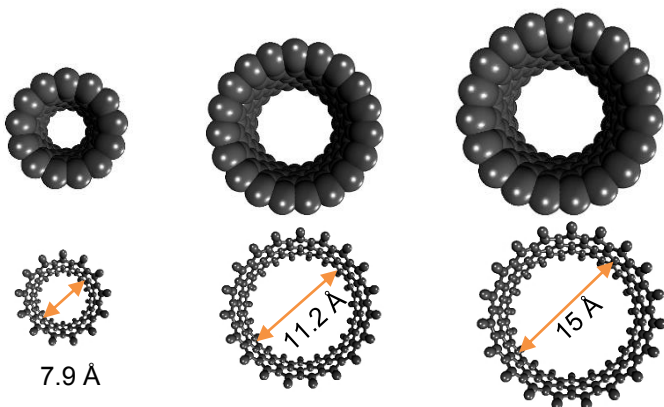
Figure 1. Schematic representation of three zigzag CNT nanostructures.
