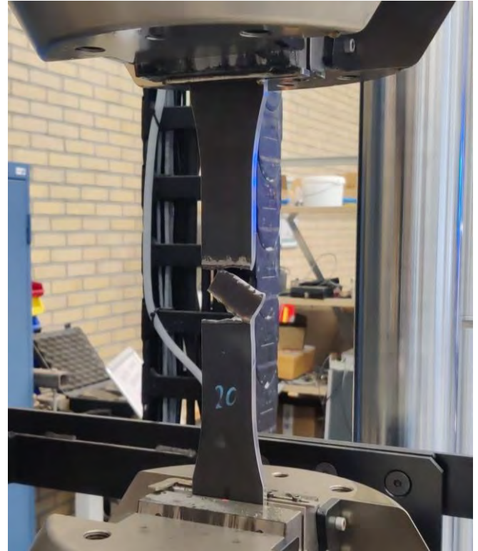
Figure 3: A friction stir welded specimen showing fatigue induced failure.
