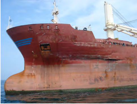
Figure 1: Damaged ship hull [1]
