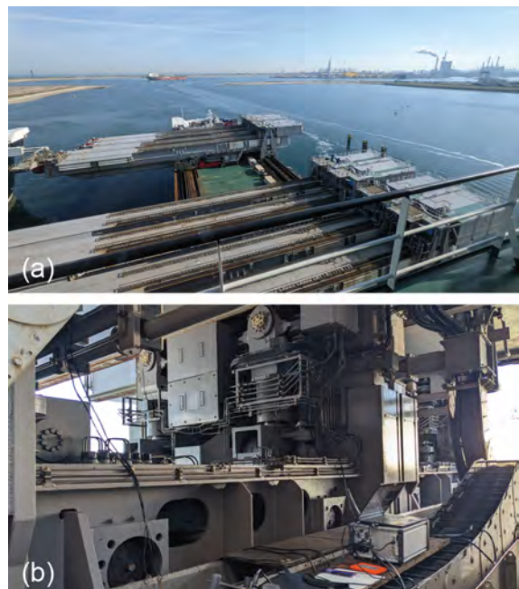
Figure 3: Pictures of "Pioneering Spirit" measurement, showing; (a) an overview of several starboard beams of the topside lift system, and (b) instrumentation of the outboard support.
