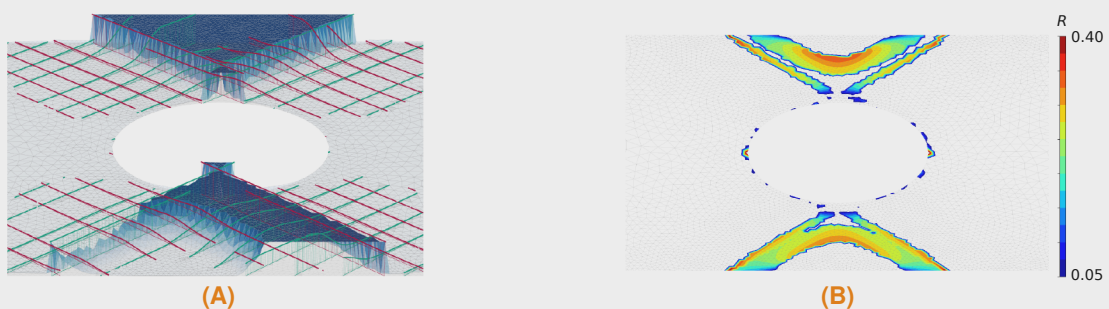
Figure 2: Results with open-hole [±45]-laminate (A) Damage evolution in XFEM cracks and interface. (B) Local stress ratio variations in the cohesive zone
