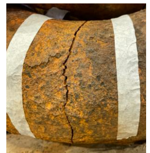
Figure 4: Main fracture in mooring chain links
