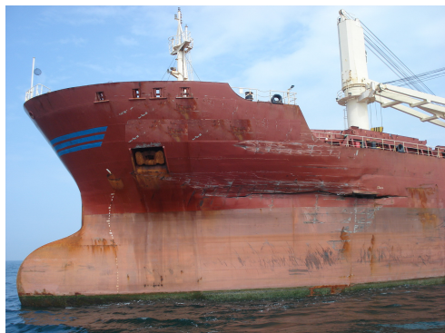
Figure 1: Damaged ship hull [1]
