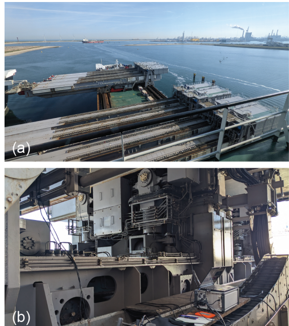
Figure 3: Pictures of "Pioneering Spirit" measurement, showing; (a) an overview of several starboard beams of the topside lift system, and (b) instrumentation of the outboard support.
