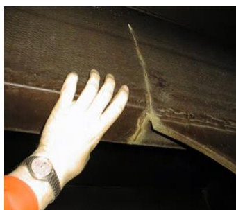
Figure 2: Fatigue crack on stiffener [1]. Figure 3: Internal ship structural frame.
