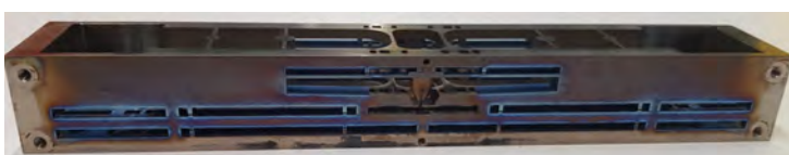
Figure 2: Vacuum compatible, monolithic, high-precision, high-capacity microbalance to measure how much material has been removed.
