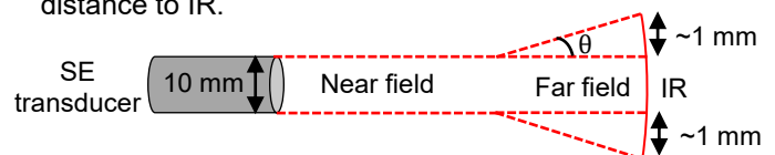
Figure 3: Near field and beam divergence of SE transducer
