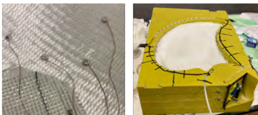
Figure 2: Left: piezoelectric sensors placed in between glass fibre laminae. Right: Laminae placed in the propeller mould [1].
