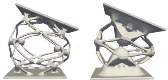
Figure 4: High-resolution three-dimensional topology optimized multi-DOF flexures for precision applications [1].
