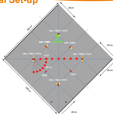
Figure 3: Experimental design (● Optics11 — FBG ● PZT)
