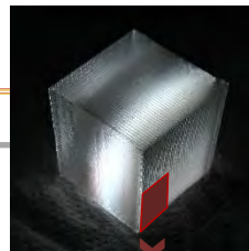
Fig. 2. \mu -CT scan image of internal structure of 3D-printed material
