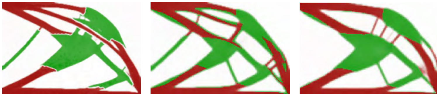
Figure 3: results for a cantilever problem, where red denotes stiff material and green compliant material. Using the conventional filter and the proposed filter with and without interface penalization
