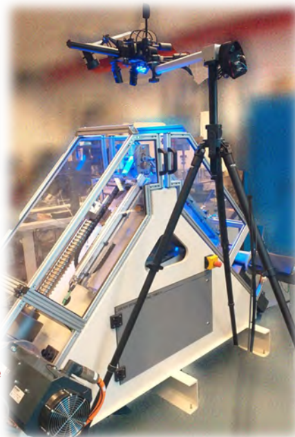
Draw-bend test and DIC setup.
