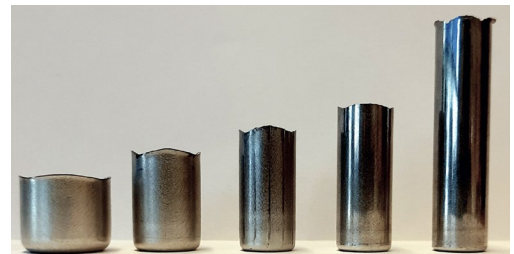
Blank at Cup-draw, Redraw-1, Redraw-2, Ironing-1, Ironing-2 stages respectively
