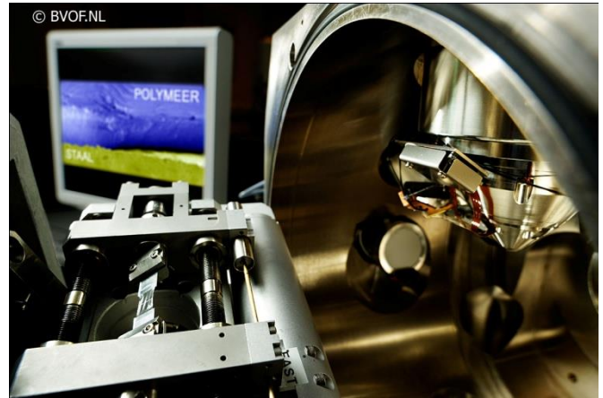
Micro-loading stage mounted in a scanning electron microscope
