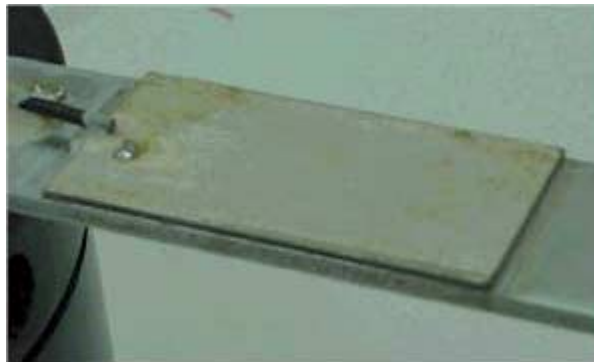
Figure 1: Piezoelectric patch bonded to a beam
